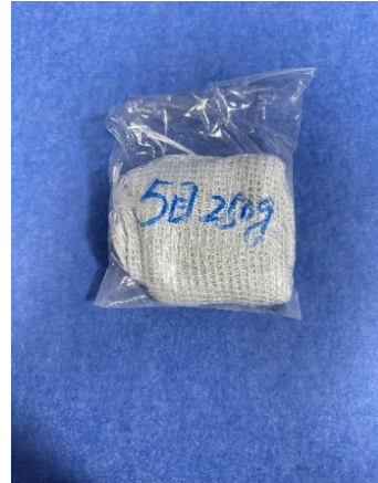
Fiberglass mesh layer (layer No.3&4&6&7)
